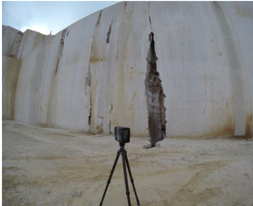
Figure 3 FARO laser scanner in operation, author photo
