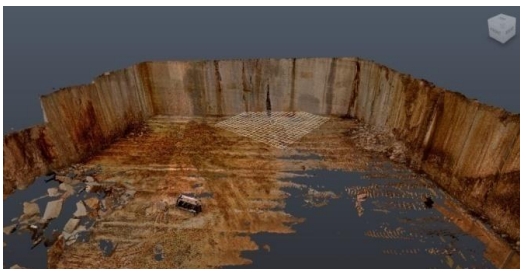
Figure 7 Obtained Point Cloud resulting from the connection of obtained individual scans – front view
